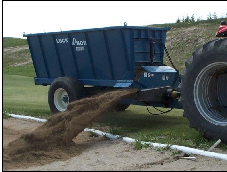
adjustable sand deflectors on discharge
