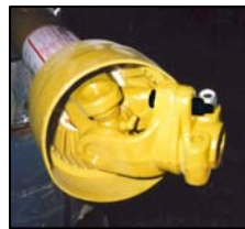
PTO drive assembly with shear bolt for equipment protection
